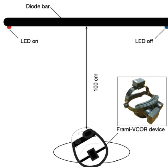
**Figure 1** Illustration of the Frami-VCOR device and setup.
